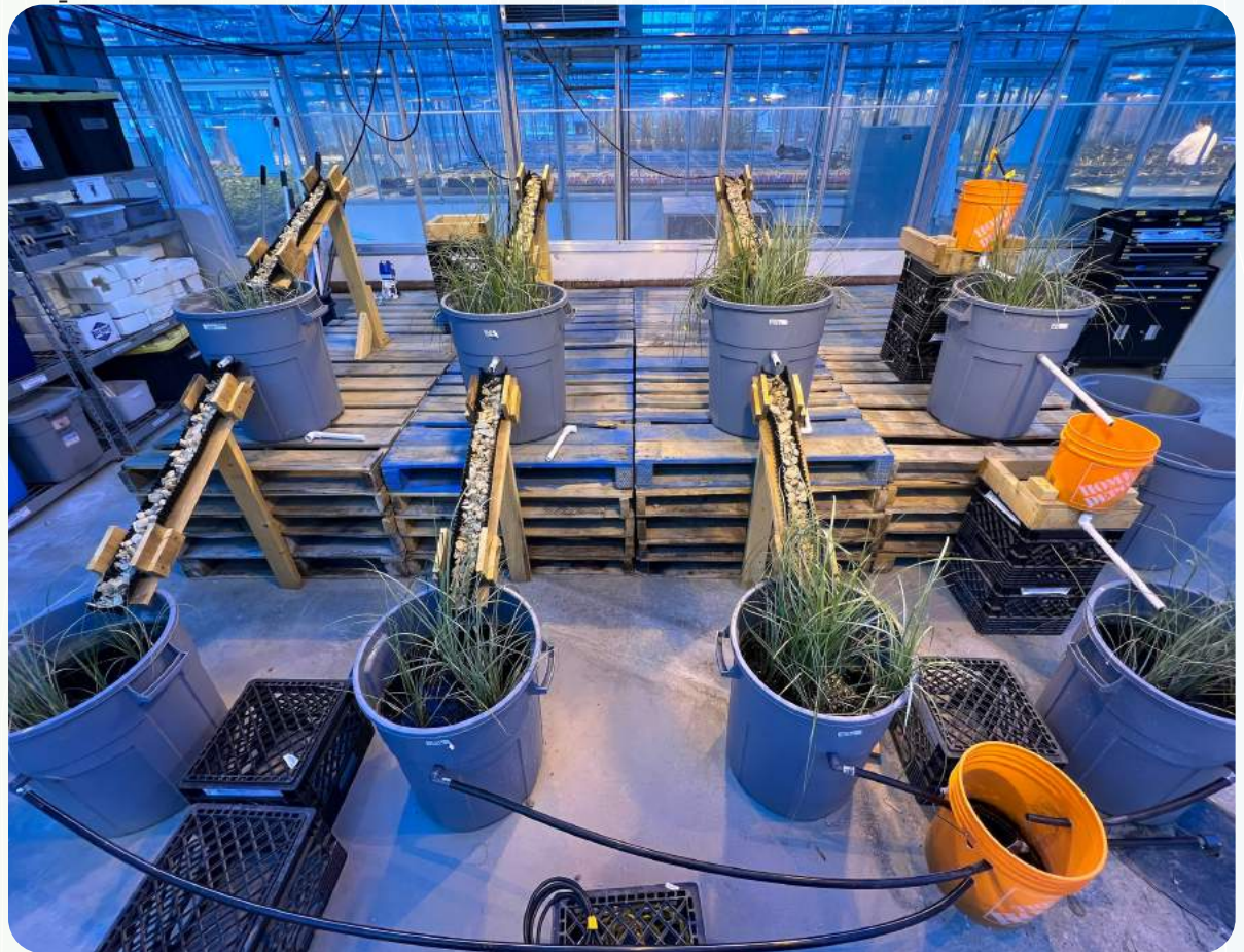
Constructed Wetland Treatment System (CWTS) bench-scale laboratory set up.
