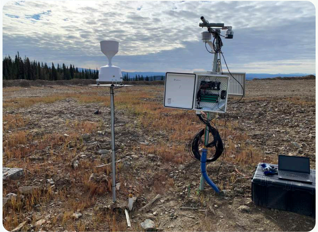
Instrumentation set up for cover monitoring on the Platinum Gulch Waste Rock Storage Area at the Eagle Gold Mine.
